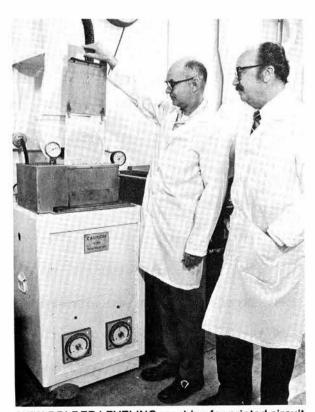
NEW SOLDER LEVELING machine for printed circuit production is demonstrated by inventors Bob Sylvester, left, and T.A. Allen (both 3623-1).
